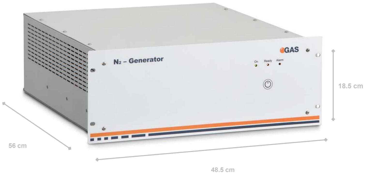
The N<sub>2</sub>-Generator of G.A.S. was particularly developed for the autonomous, mobile and by that flexible use of analytical devices where zero air is no option e.g. testing of flammable gases. Using the N<sub>2</sub>-Generator makes cylinders of operating gas redundant allowing analyzers to be operated continuously with nitrogen of highest grade (5.0) supplied from enriched ambient air.
