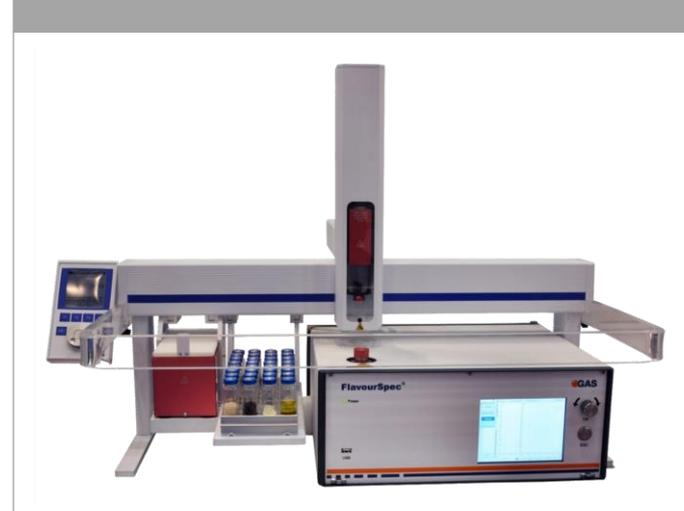
The FlavourSpec made by G.A.S. offers a gas-chromatographic separation and high sensitive detection via ion mobility spectrometry. The automated built-in agitator and coupled autosampler enable an efficient and fast workflow.
