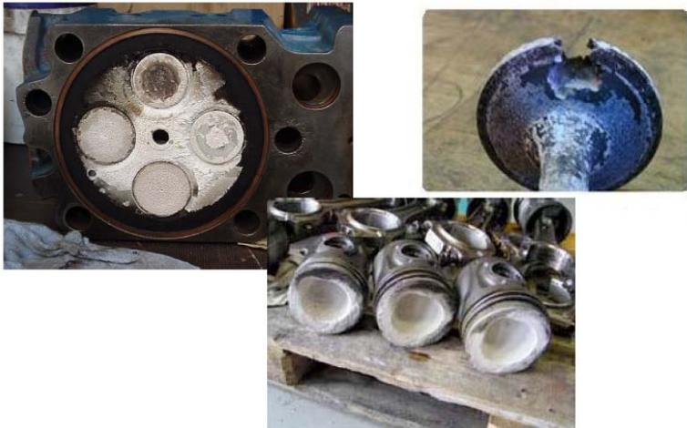
Figure 2: Defects on engine parts due to silica
