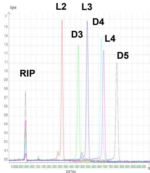
Figure 4: IMS spectra of individual siloxanes
