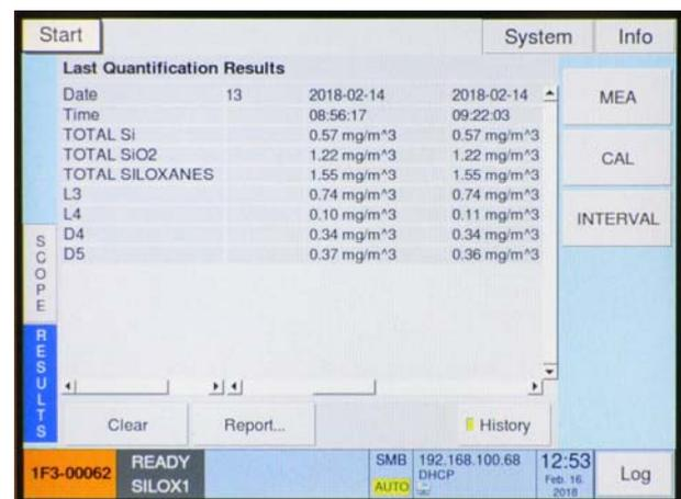
Figure 5: GC-IMS-SILOX result window. L2, L4 and D4, D5 are displayed same as the calculated concentration for total siloxanes, silica and silicon.
