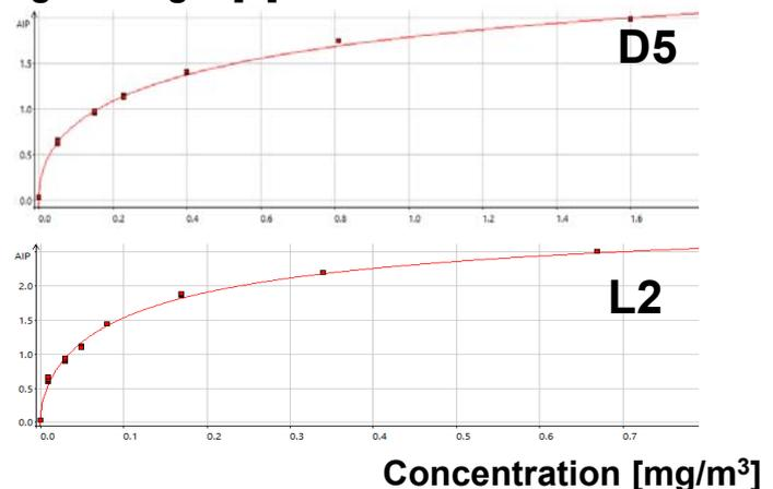
Figure 6: By using certified permeation tubes and sophisticated gas-dilution various headspace concentrations of the siloxanes are achieved to create a calibration curve; e.g.: D5, L2
