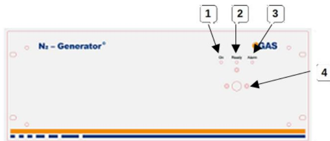
During normal operation the **red LED (3)** is OFF and the system carries out several automatic checks.
