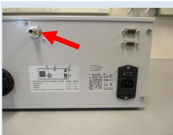
Connect the output to the device input (Drift gas/Carrier gas adapter) using a 3 mm (Swagelok) tube.
