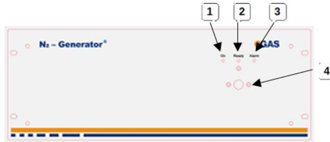
The front panel has **three LEDs**: **GREEN (1)**, **YELLOW (2)**, **RED (3)** and **START/STOP button** (4)
