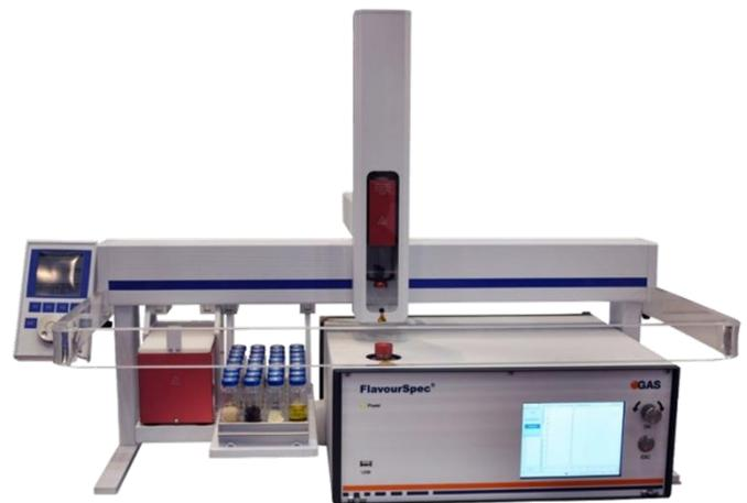
**Figure 5:** The FlavourSpec made by G.A.S. offers an orthogonal separation by gas-chromatography and ion mobility spectrometry while the latter is used as detector at the same time. The built-in agitator and coupled autosampler enable an efficient and fast workflow.
