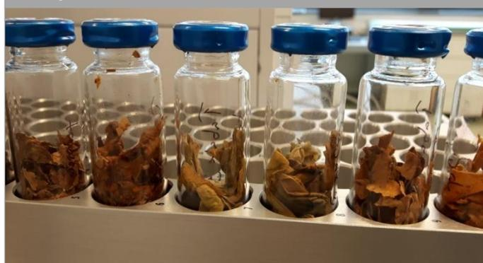
**Figure 1:** A small amount of tobacco leaves was directly transferred into the headspace vial. A further sample pre-treatment is not necessary.
