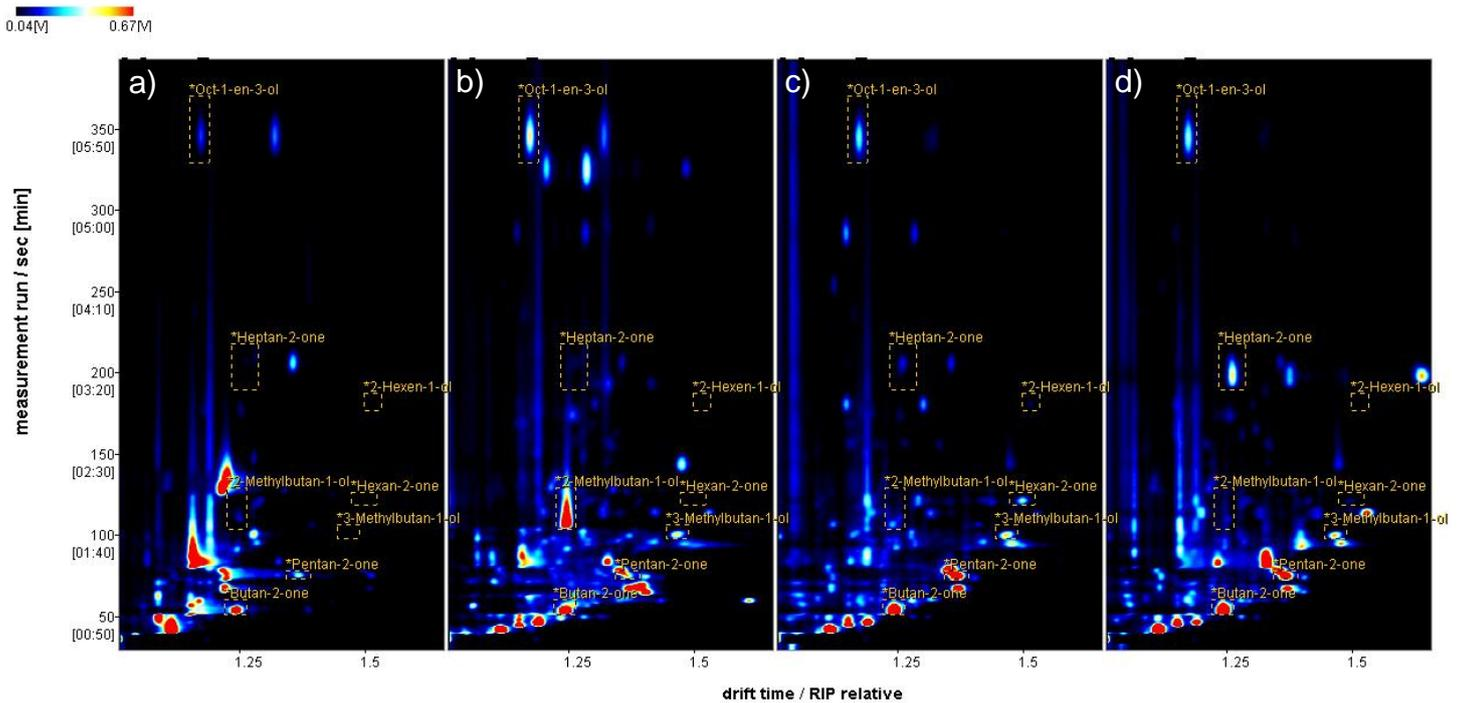
**Figure 3:** GC-IMS headspace measurements of moulded tobacco leaves. Potential funghi markers are marked (dashed yellow rectangle). Brazil-Dark Air Cured (a), India-Sun Air Cured (b), Brazil-Flue Cured Virginia (c), Malawi-Burley (d).
