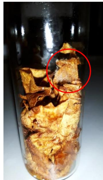
**Figure 2:** Sample as-is after moistening and 10 days incubation. The generated mycelium can be clearly seen (red circle).
