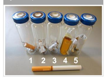
The cigarette and packaging samples were directly transferred into the headspace vial. A sample pretreatment is not necessary.
