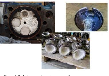
Figure 2: Defects on engine parts due to silica
