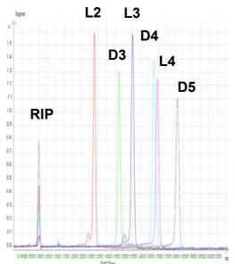
Figure 4: IMS spectra of individual siloxanes
