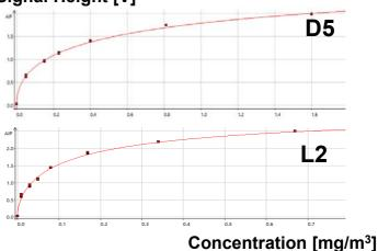
**Figure 6:** By using certified permeation tubes and sophisticated gas-dilution various headspace concentrations of the siloxanes are achieved to create a calibration curve; e.g.: D5, L2
