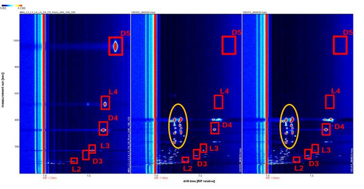
Figure 7: 3 GC-IMS chromatograms of landfill gas
