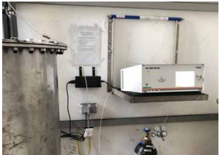
Figure 3: GC-IMS-SILOX on-site at a landfill site
