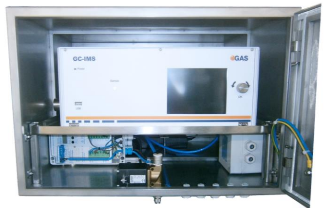
Figure 4: GC-IMS instrument for monitoring of TICs in chemical plants embedded into a pressurized enclosure system. The pressurized enclosure system ensures safety class Ex II 2 G Ex px II T4 (German Explosion Protection Ordinance).
