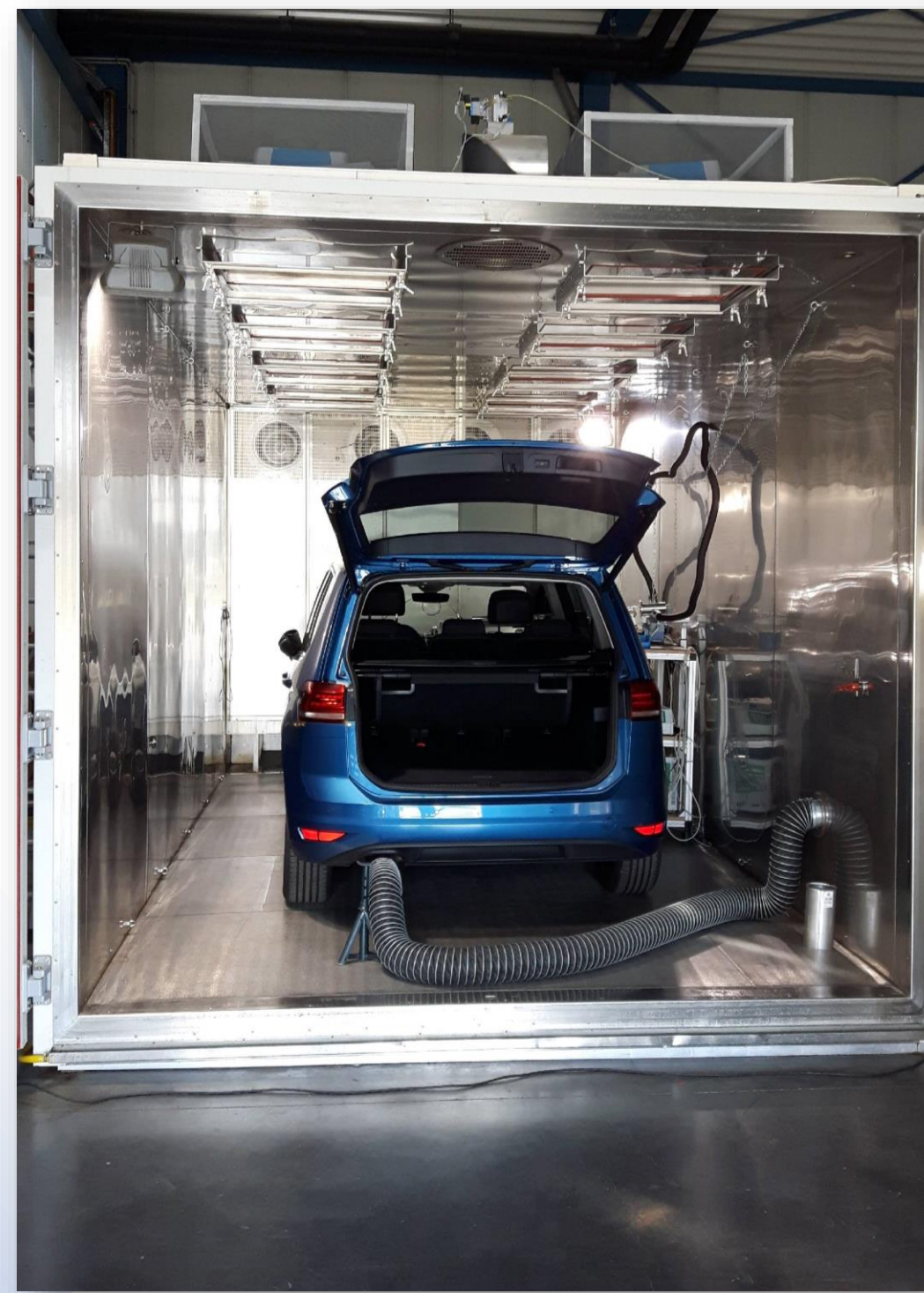
Exemplary picture of measurement chamber. Different vehicles were located in the temperature, radiation and humidity controlled measurement chamber based on ISO standard 12219-1.
