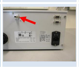
Connect the output to the device input (Drift gas/Carrier gas adapter) using a 3 mm (Swagelok) tube.
